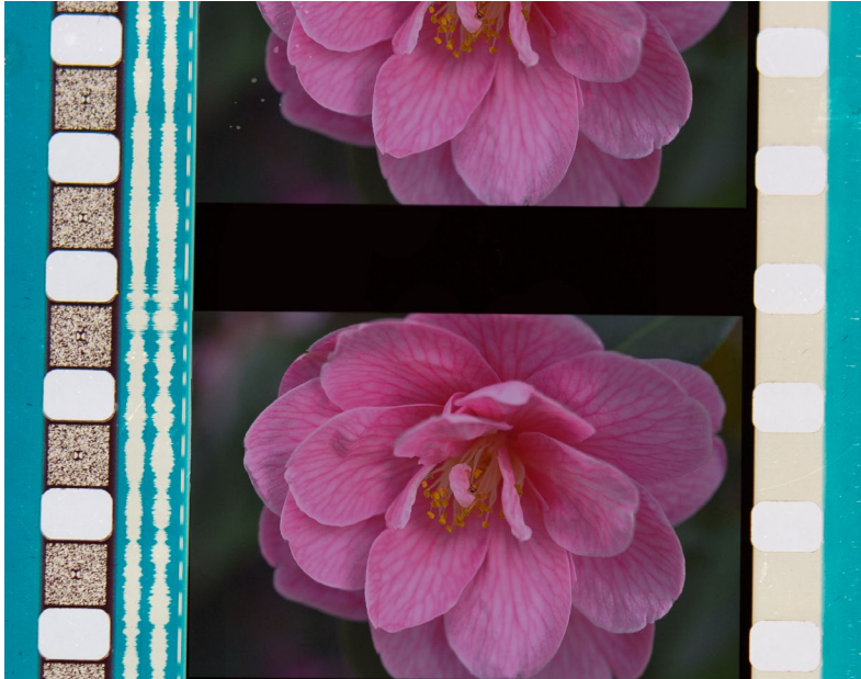
A close up of film frames with a: optical variable area track, a Dolby Digital track (situated between the perforations) and a DTS track (intermittent line next to film image)
